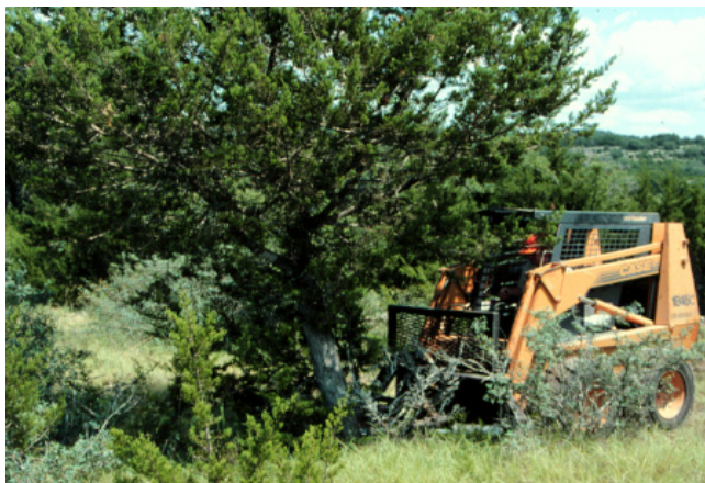
Figure 10. A base shearer being used on juniper. Photo by Richard B. Taylor.
