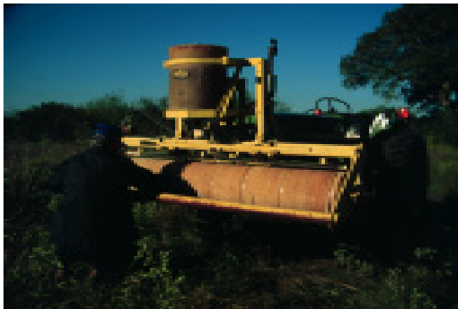
Figure 14. A carpet roller is one method of foliar application of herbicides. Photo by Timothy Fulbright.
